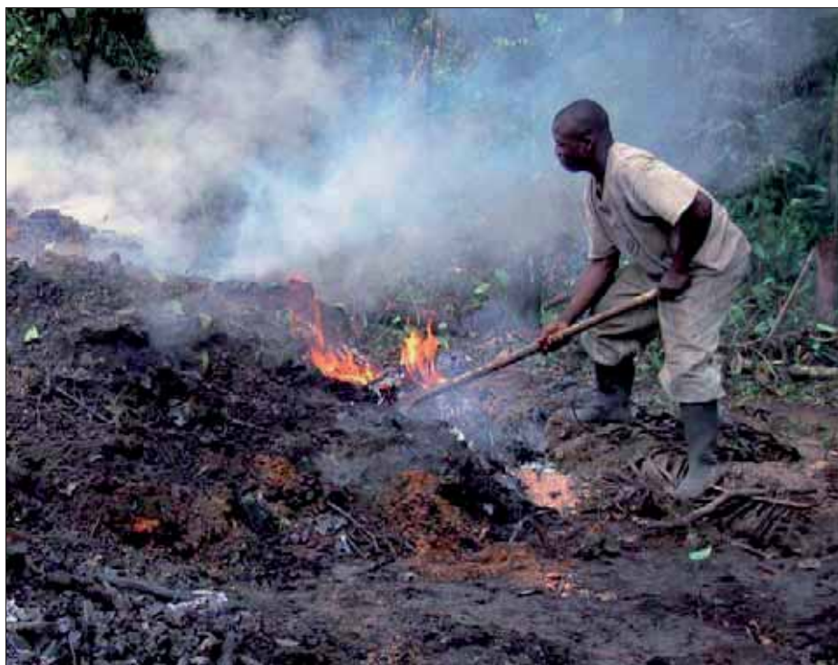
In many places, including Liberia, charcoal is produced using simple earth pits
